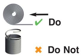
Do not twist the cable when unwinding. always unwind straight from spool.
