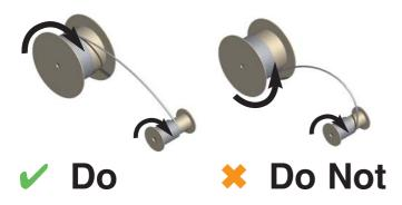
Ring put ups require careful uncoiling by rolling the ring upright over the floor
