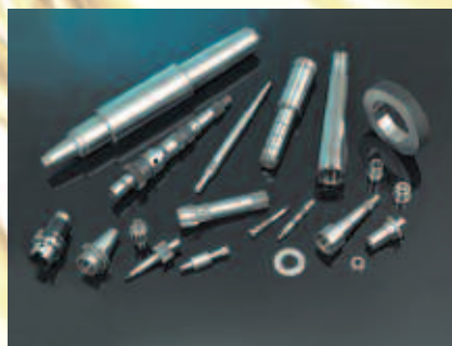
Pins, axles, sockets, nozzles and other parts are manufactured on Studer cylindrical grinding machines.
